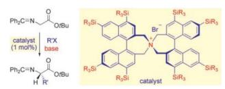
**Designer rings**: Chiral phase-transfer catalysts with 4,4′,6,6′-tetrasubstituted binaphthyl units give excellent enantioselectivity in the asymmetric alkylation of *tert*-butylglycinate—benzophe-
